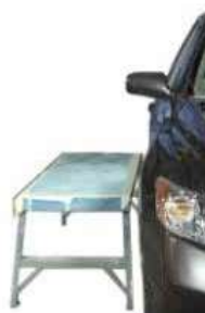
A platform allows the worker to position himself at the right height. Markers can be placed on the side to avoid scratching the vehicle.
